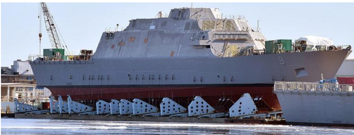
Fig.45. the positions of slip truck depend on the length of the ship [27]
