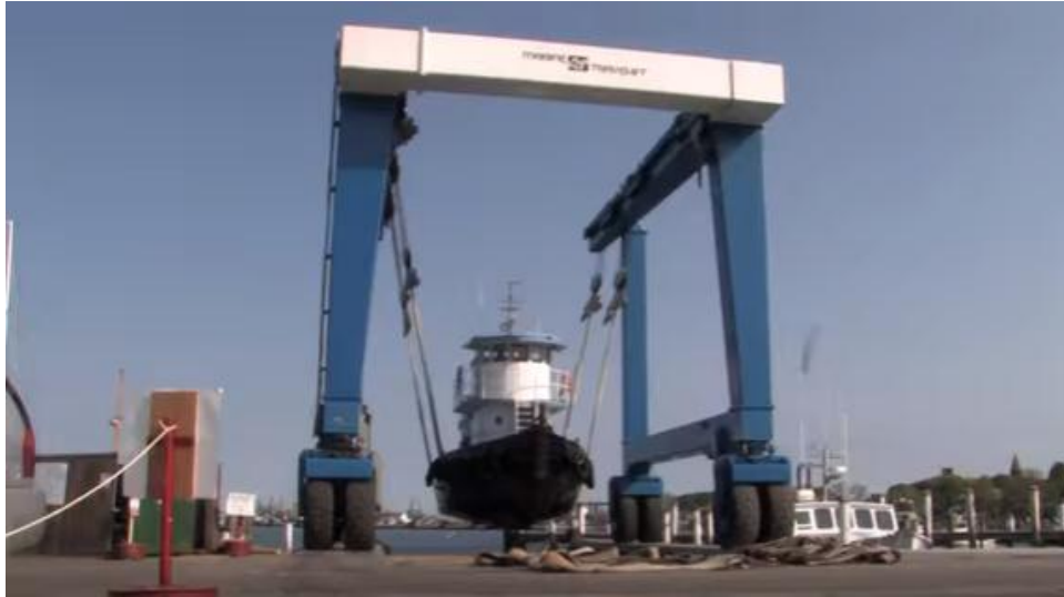
Fig.9. Ship launching by Travel lift [15]
