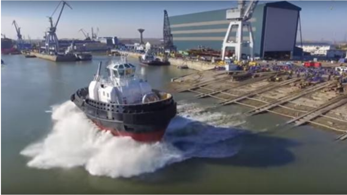
Fig.14. Transversal launching in slipway [9]
