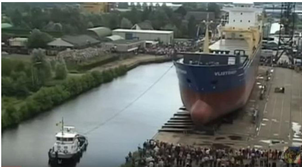
Fig.16.Normal ship launching from slipway of river shipyard [9]
