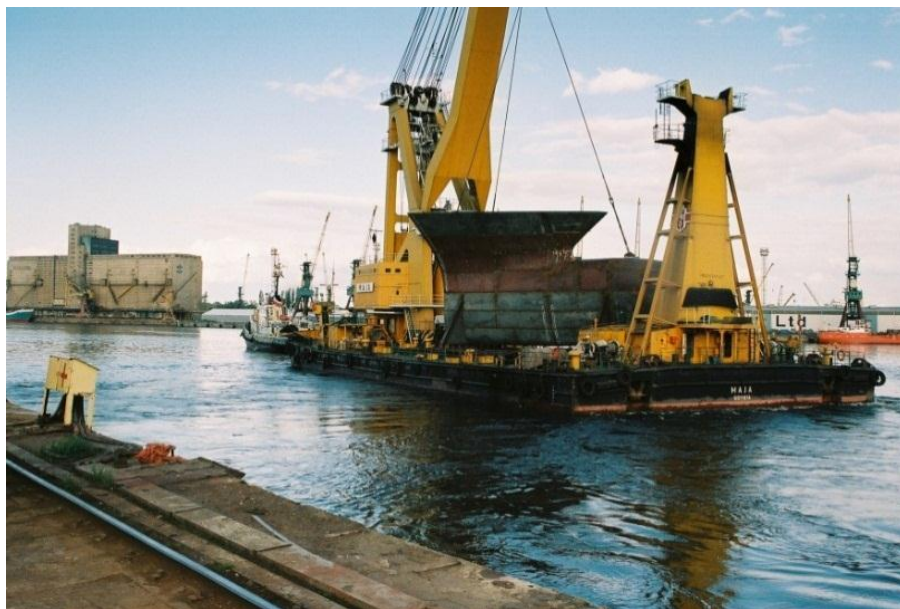
Fig.20. Transport of ship block, by floating crane [14]
