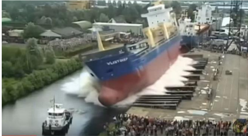
Fig. 17. Leap Launch of ship, in close water way (Canal) [9]
