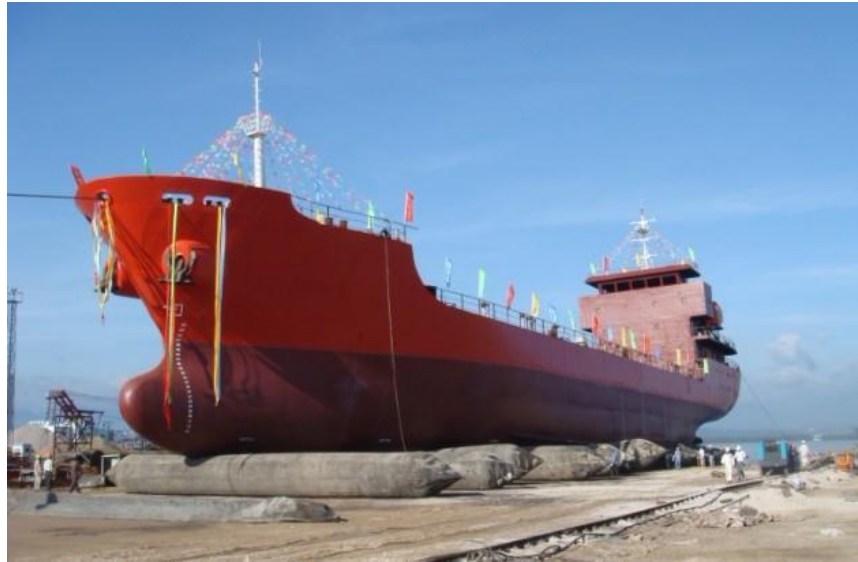
Fig.5. Ship launching in airbags [10]
