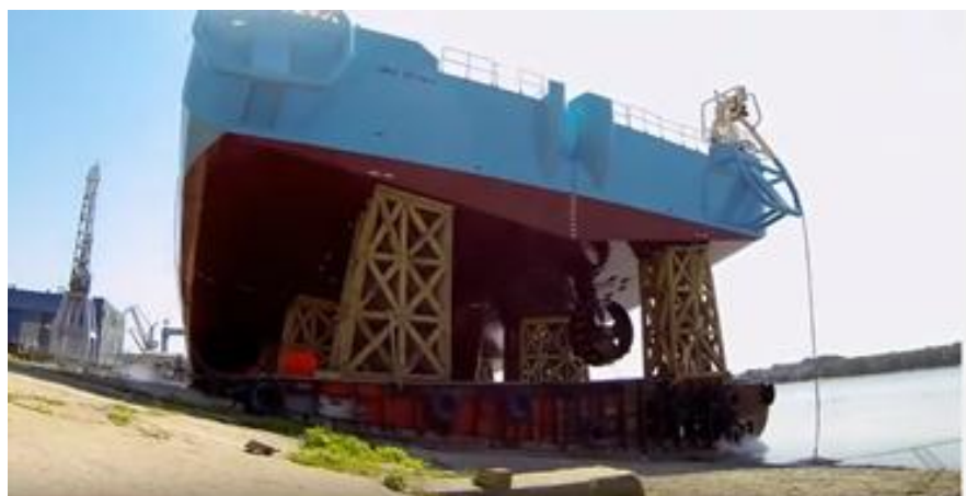
Fig.16.Normal ship launching from slipway of river shipyard [9]
