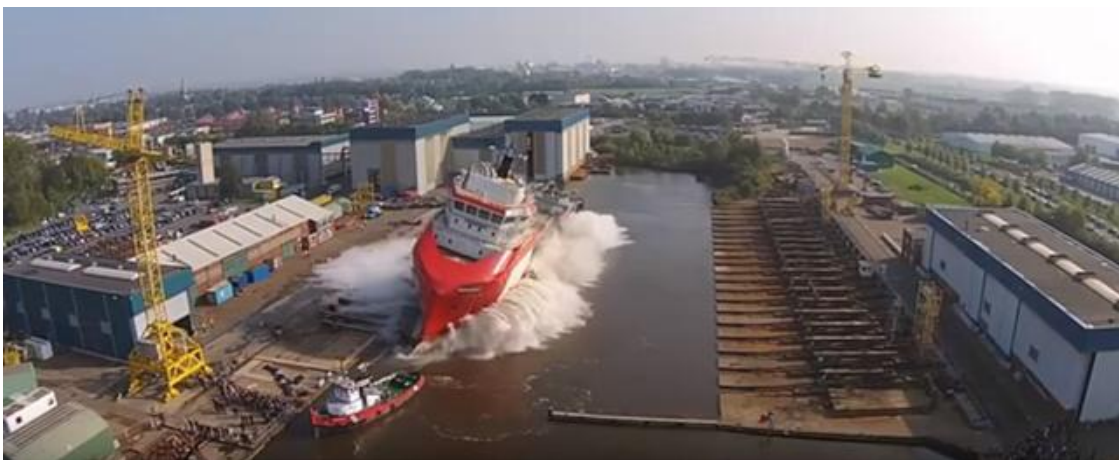
Fig.4. Transversal ship launching in canals [9]
