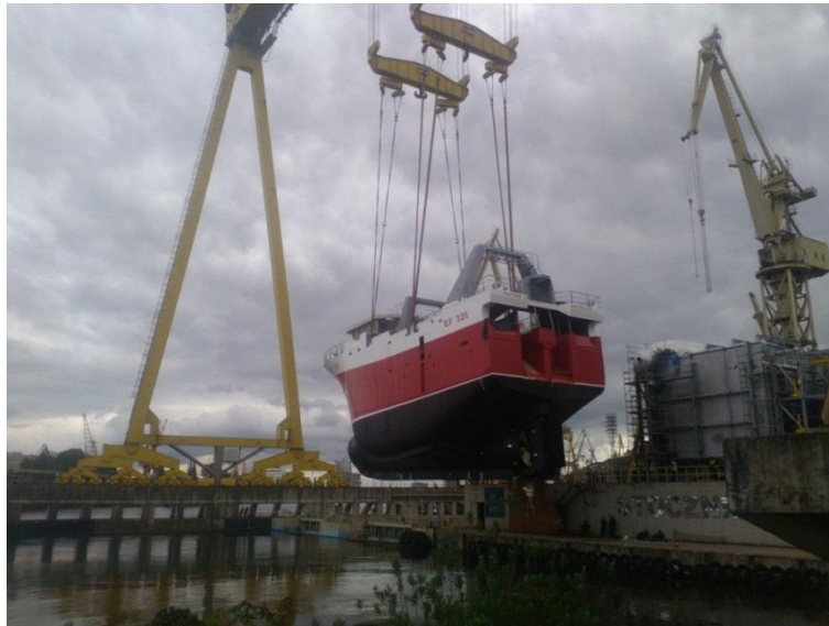
Fig.21.Ship launching by crane is shipyard [14]
