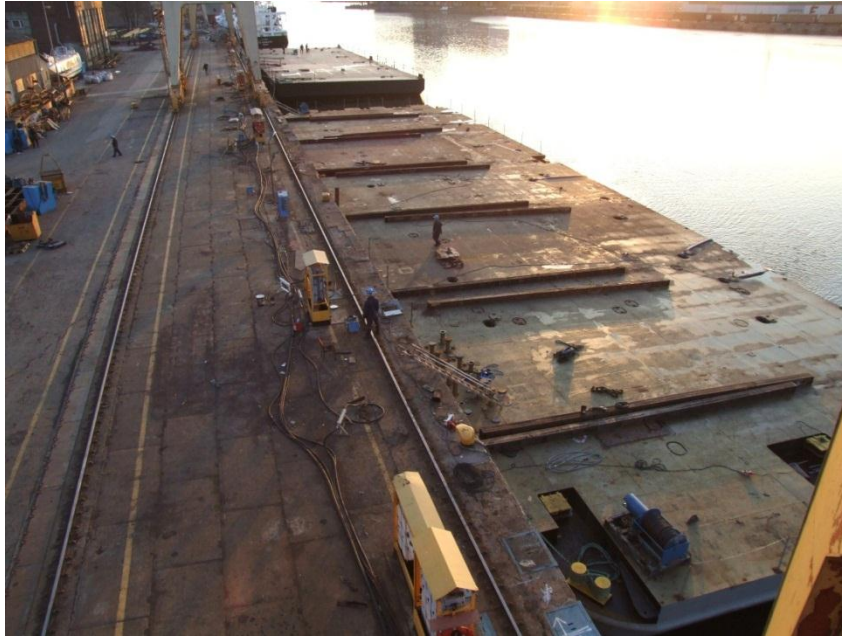
Fig.38. Pontoon in statically position for making the transfer of ship [14]
