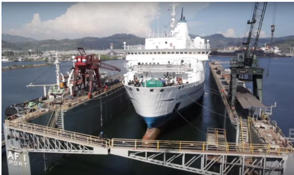
Fig.7.Ship launching by floating dock [13]
