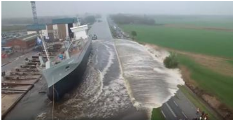
Fig.22 interruption of transit caused by the waves made for the launch process [9].
