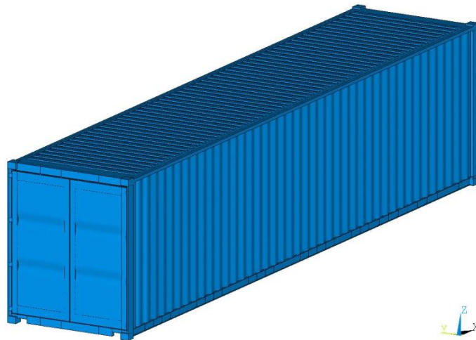
Figure 4.1 – FEM model of the 40-foot HQ container modelled with shell elements.
