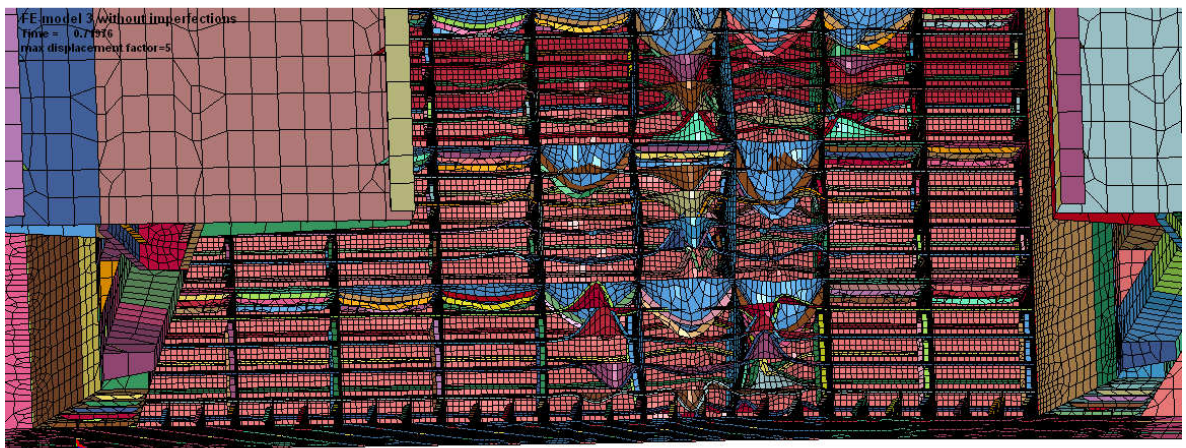
Figure 48 Deformation of the bottom girders
