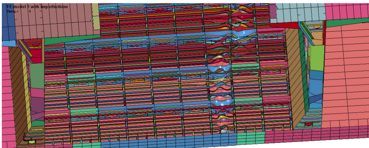
Figure 58 Deformation in the side girders in the double bottom
