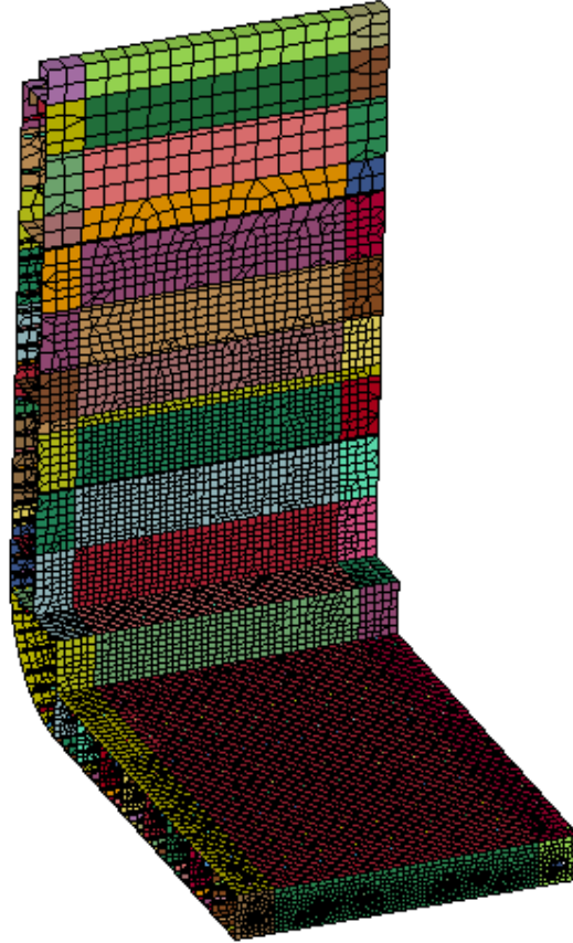
Figure 98 Mesh nr 2 generated on the container ship model
