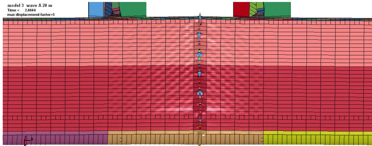
Figure 82 Deformation of the outer bottom structure
