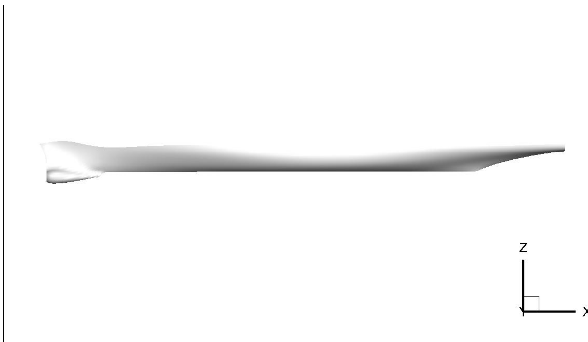
Fig. 5 Geometry of DTMB 5415
