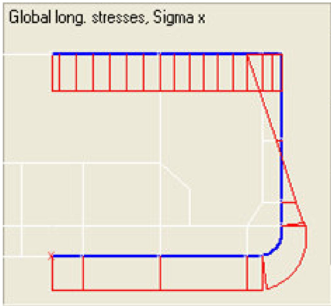
Figure 4.17 Global longitudinal stress in sagging at mid ship section
