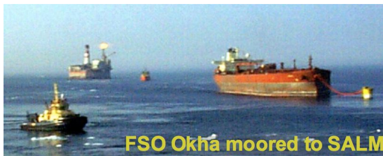
(c) FSO tanker escorted up to, and then moored at a SALM buoy [3] [5]
