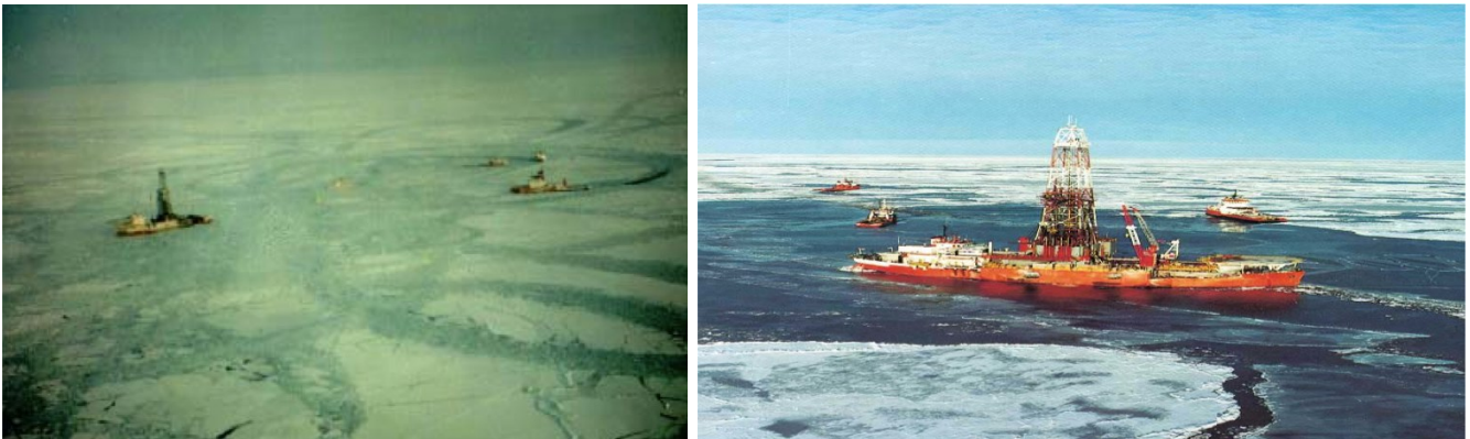
(a) Ice management around a moored drilling vessel [3]
