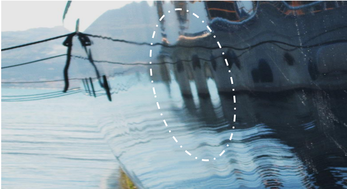
Figure 2: Image of the port side of a motor yacht with an aluminium hull, showing warping-distortions seen along the longitudinal direction, due to uneven thermal expansions
