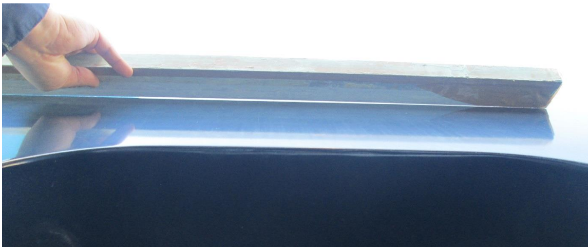
Figure 58: Visible gap over a porthole clearly visible (midships)
