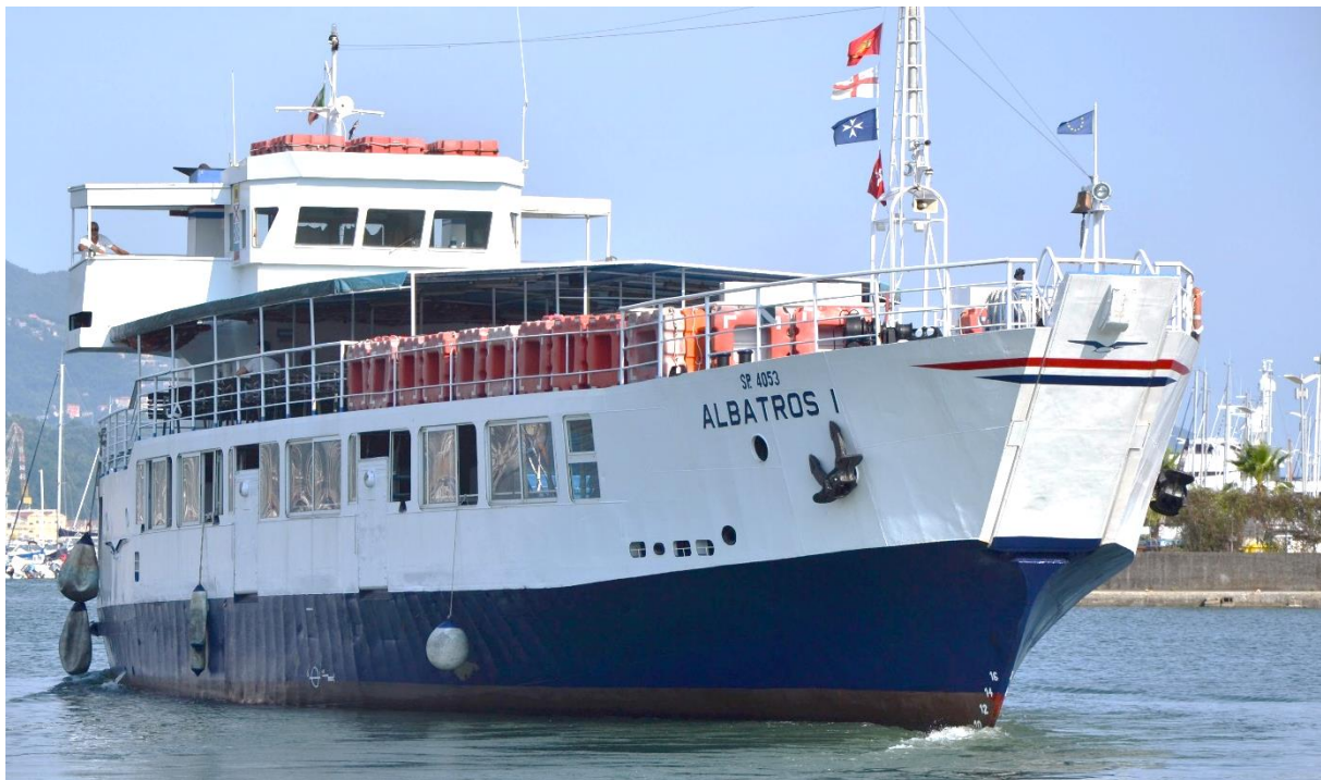
Figure 4: Image of a ferry (taken at the marina) without any epoxy filler layers. Deflections are clearly visible in the blue painted region and justify the need for epoxy layering (taken in Aug, 2013)
