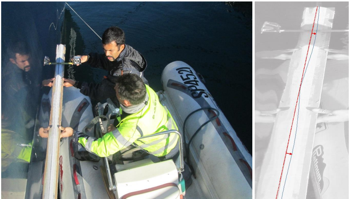
Figure 56: Image showing the author (in black jacket) measuring deformations from a boat
