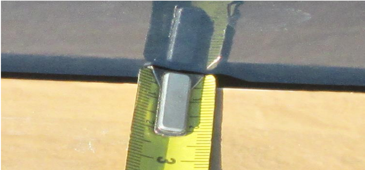
Figure 55: Scale measurement of deflections in between two transversal frames
