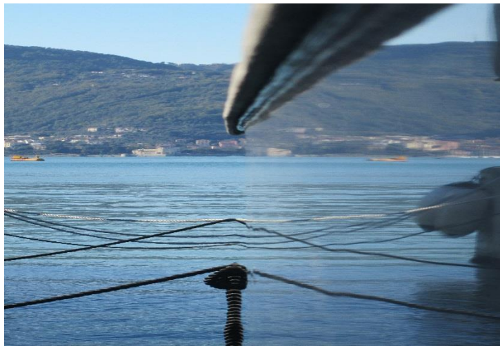
Figure 64: Surface imperfections can be easily seen in above image where the smooth lines of the mooring lines appear jagged and wavy in the reflections on the yacht's surface
