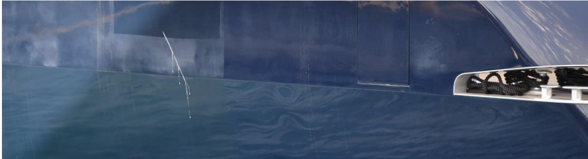
Figure 72: Paint defects due to thermal creep and over-curing in the epoxy-paint layer interface
