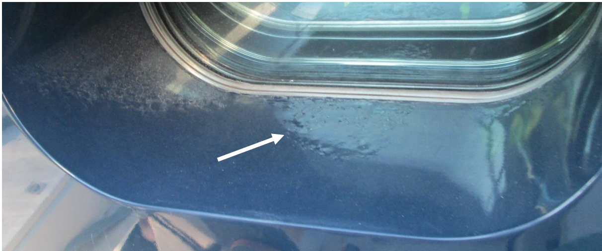
Figure 73: Paint de-bonding effects due to strong focussing of sunlight on the paint surface
