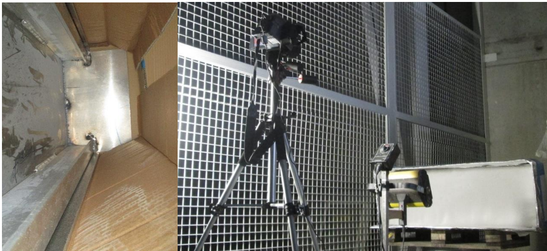
Image (left) shows the back panel covered to reduce radiation and natural convection (as in a ship) while image (right) shows the setup of the thermal imaging camera and the halogen lamp.
