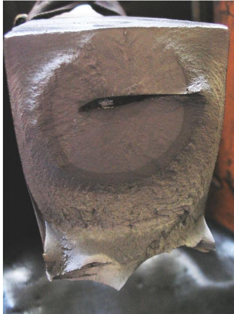
Figure A. 28. Fatigue crack surface of specimen up5 (elliptical embedded crack)
