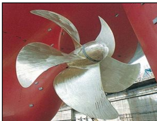
Figure 10. Fixed Pitch Propeller of a merchant ship.
