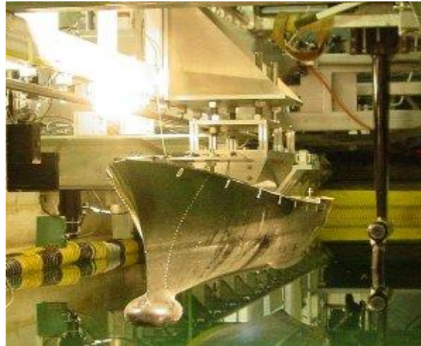
Figure 20: Model 5512 suspended in air from the IIHR towing tank carriage
