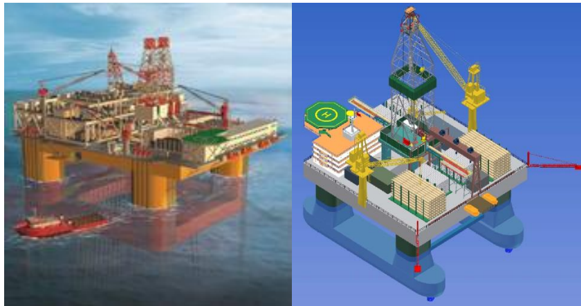
Figure 12 Column Stabilized Semisubmersibles (Left: Ring Pontoon Design, Right: Twin Pontoon Design, Source: Petrowiki)
