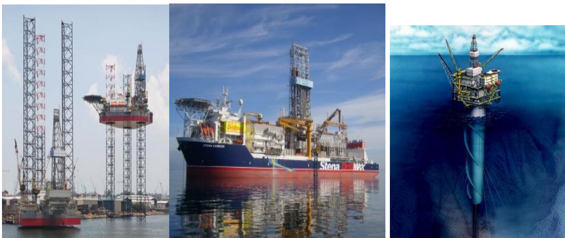
Figure 8 Jack-up drilling rigs (Left, Source: www.worldmaritimeneews.com ), Drill ships (Middle, Source: www.dft.gov.uk ), Spar Platform (Right, Source: www.marineinsight.com )
