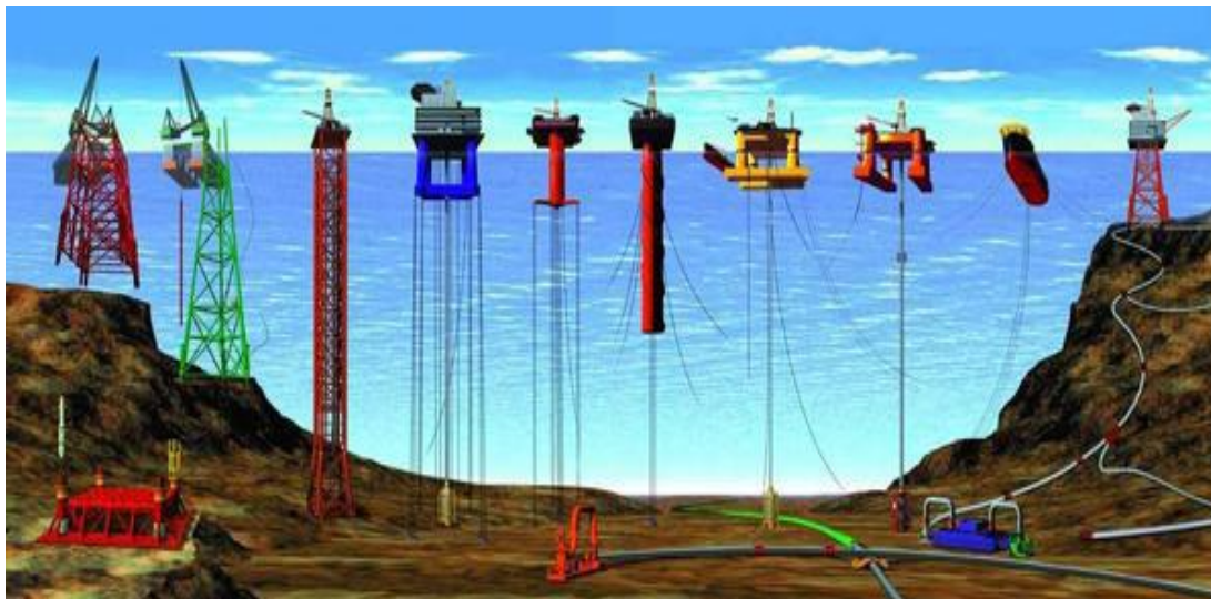
Figure 5 Types of Offshore oil and gas structures (from left to right) : 1, 2) conventional fixed platforms 3) compliant tower (4, 5) vertically moored tension leg and mini-tension leg platform 6) Spar (7,8) Semisubmersibles 9) Floating production, storage, and offloading facility; 10) sub-sea completion and tie-back to host facility (Source:www.oceanexplorer.noaa.gov)
