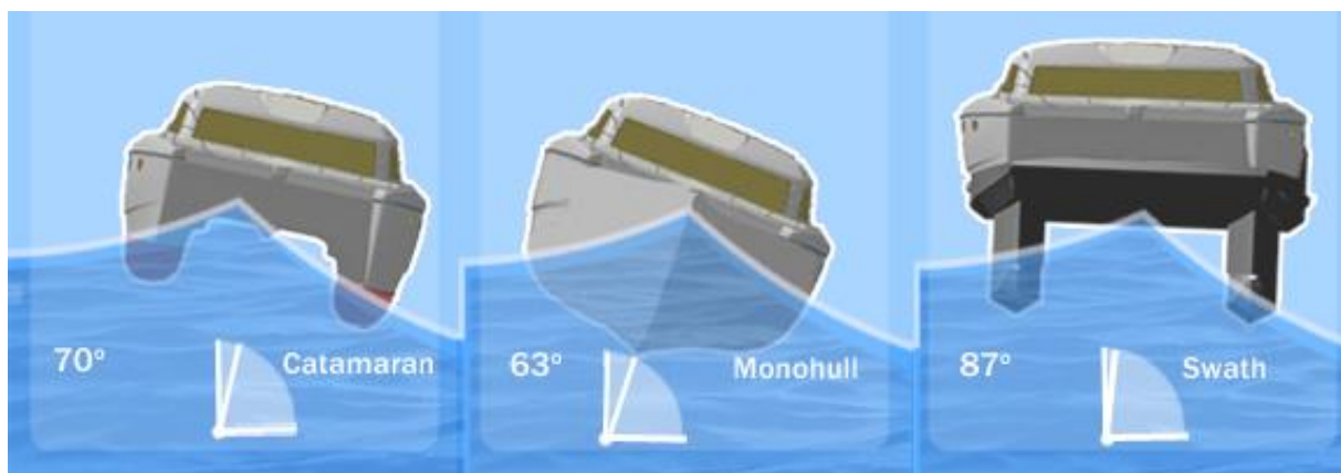
Figure 6 : Rolling angles response of a six foot wave [www.stabilityyachts.com, 01/06/13]
