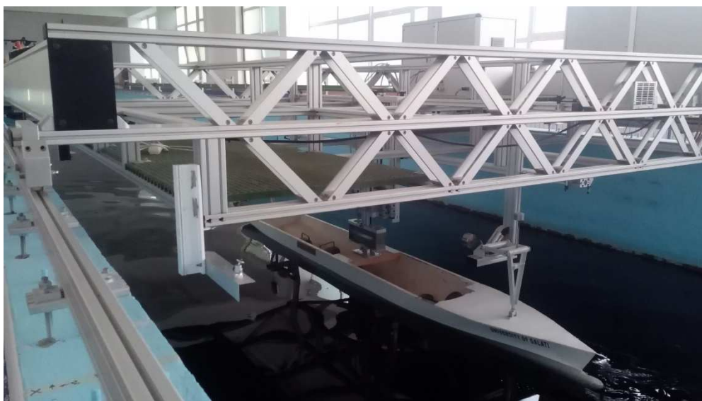
Figure 45. The KCS model during the resistance test.
