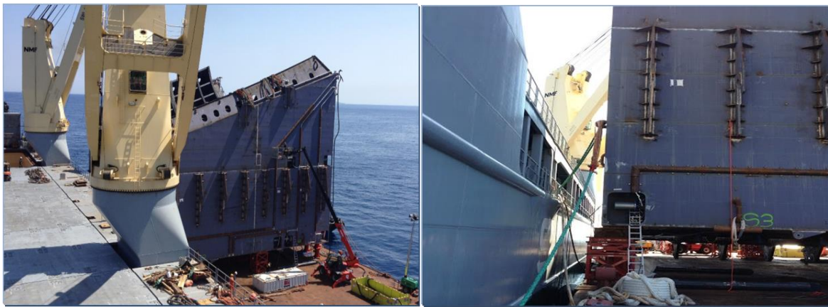
Figure 4- 5 A heavy lift vessel and a transport barge during cargo transfer operation : Topview (left) & The gap (right). (Source of photoes: SAL Heavy Lift)
