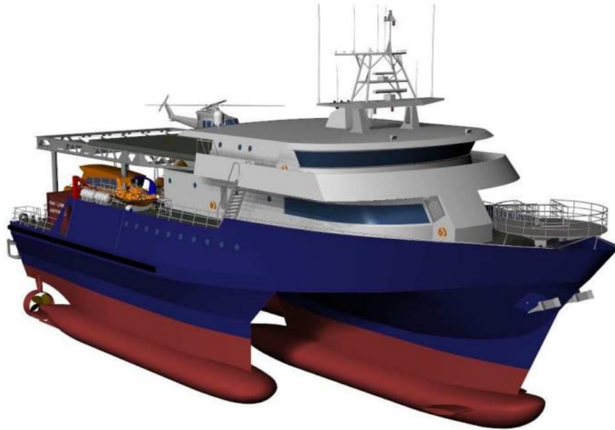
Figure 2 MAURIC wind farm support mother Vessel WSMV computer rendering Source: Bureau Mauric
