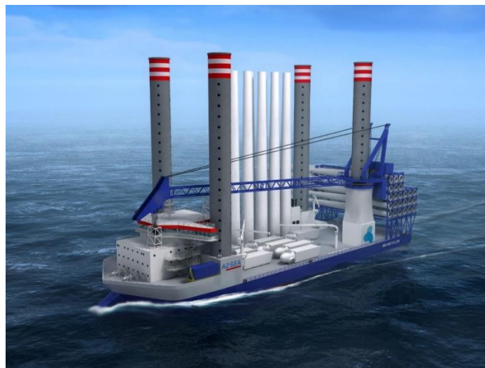
Figure 41. Example of WTIV during transient phase and cargo on deck.
