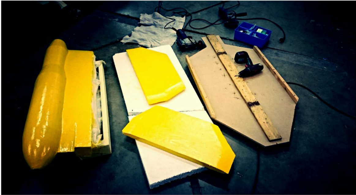
Figure 6.18 Central Hull, Outriggers (coated with resin and painted) along with Wooden Deck
