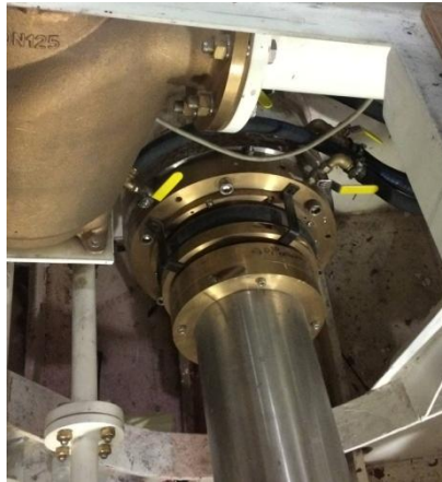
Figure 43. Deep sea seal on actual ship in construction "Pachamama". Picture taken at Baglietto's Shipyard, La Spezia, Italia.
