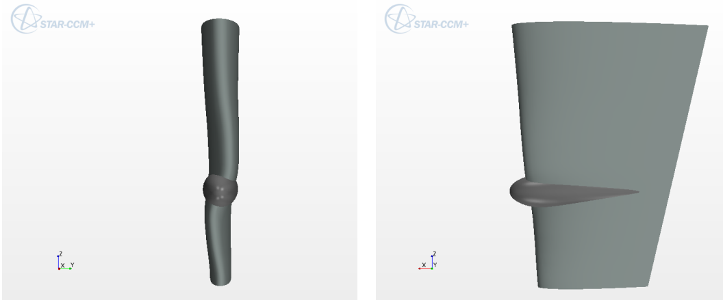
Figure 3.3.: Twisted Rudder modelled in CAESES framework
