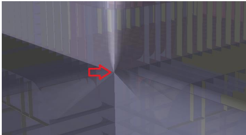
Figure 6-25 Area not considered in the fatigue analysis
