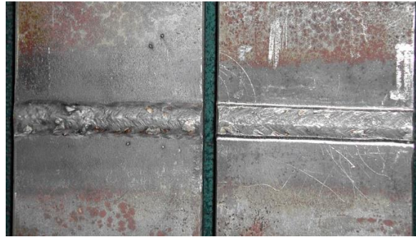
Figure 9-5 The view of the butt welds in as-welded condition (left side sample) and after application of UP (right side sample). Available in http://www.sintes.ca/Ultrasonic-Impact-Treatment.php
