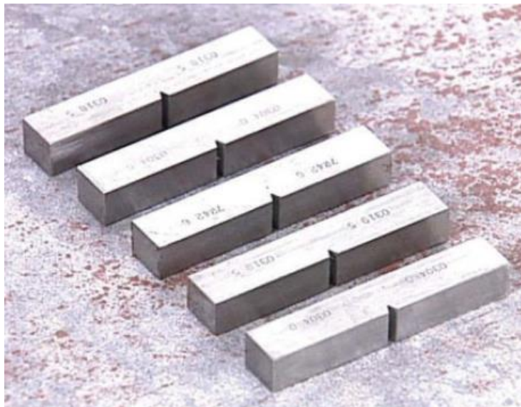
Figure 12: Charpy V-notch test specimen. Available from Hobart Institute of Welding Technology (2010)
