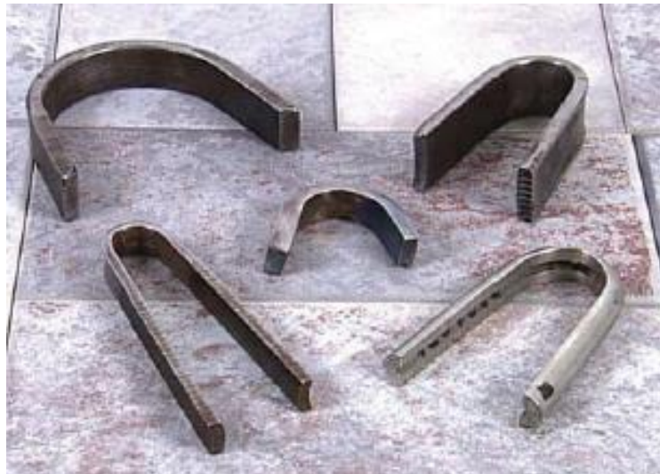
Figure 13: Bend test sample specimen. Available from Hobart Institute of Welding Technology (2010)
