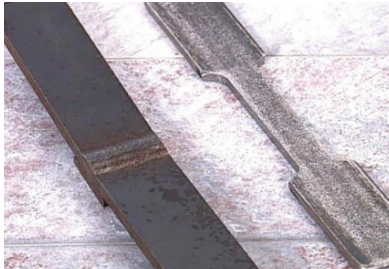
Figure 11: Tensile test specimen before and after machined to perform reduced tensile test. Available from Hobart Institute of Welding Technology (2010)
