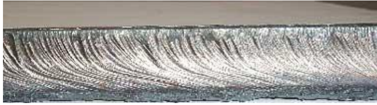
Figure 3.30 Cutting Too Fast
