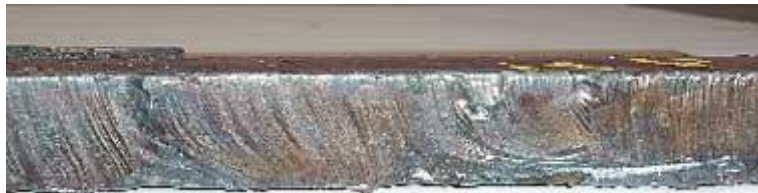
Figure 3.32 Too High Oxygen Flow
