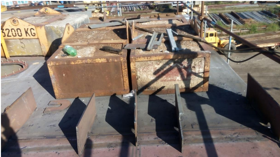
Figure 3.61 Straightening by heavy weight
