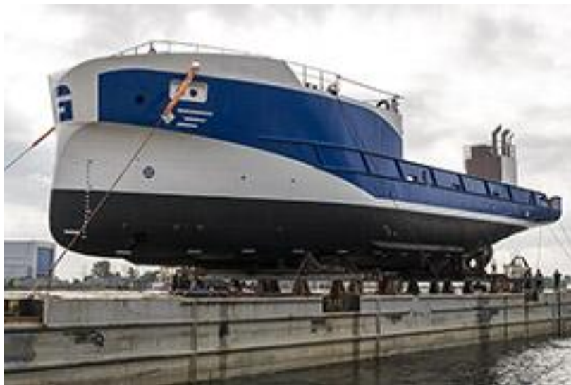
Figure 3.80 Process of launching ship by pontoon and hydraulic pistons
