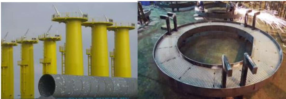
Figure 3.93 Foundations for towers for wind power plants
