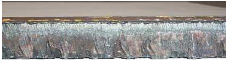
Figure 3.31 Too high nozzle to plate distance
