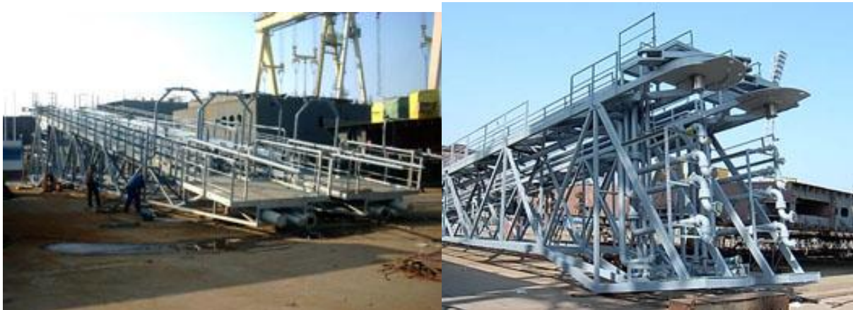
Figure 3.83 FINOMAR product burner boom
