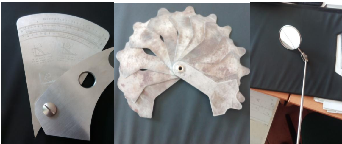
Figure 3.50 Fillet gauges measures
