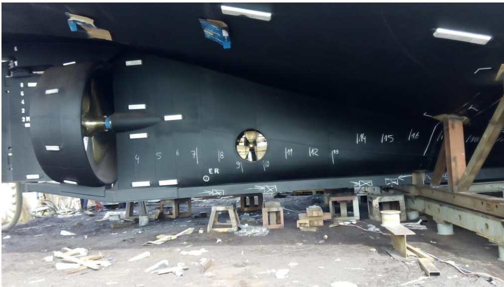
Figure 3.72 Distribution of sacrificial anode on hull of ship
