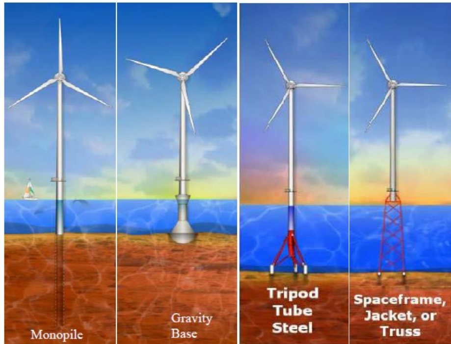
Figure 16: Shallow and deep-water foundation technologies (Aydin 2007)
