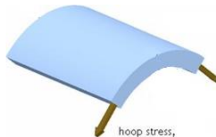
Figure 40: Hoop stress on the structure (“EngrApps: Burst and Collapse - Pressure Vessel Design” n.d.)
