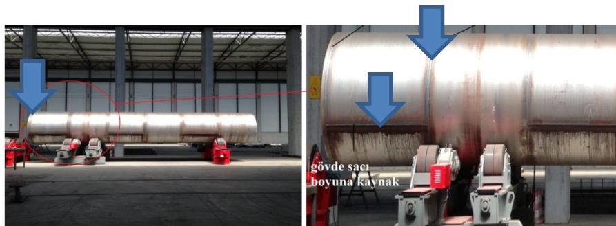
Figure 45: Welding connections in the tower (Kanbur 2014)
