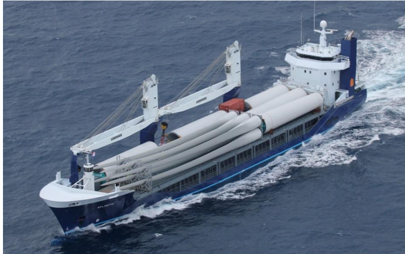
Figure 21: Tower and blades transportation for offshore wind turbines (“Heavy Lift Vessel ‘Atlantic’ Delivered to Her Owners - CONOSHIP” n.d.)
