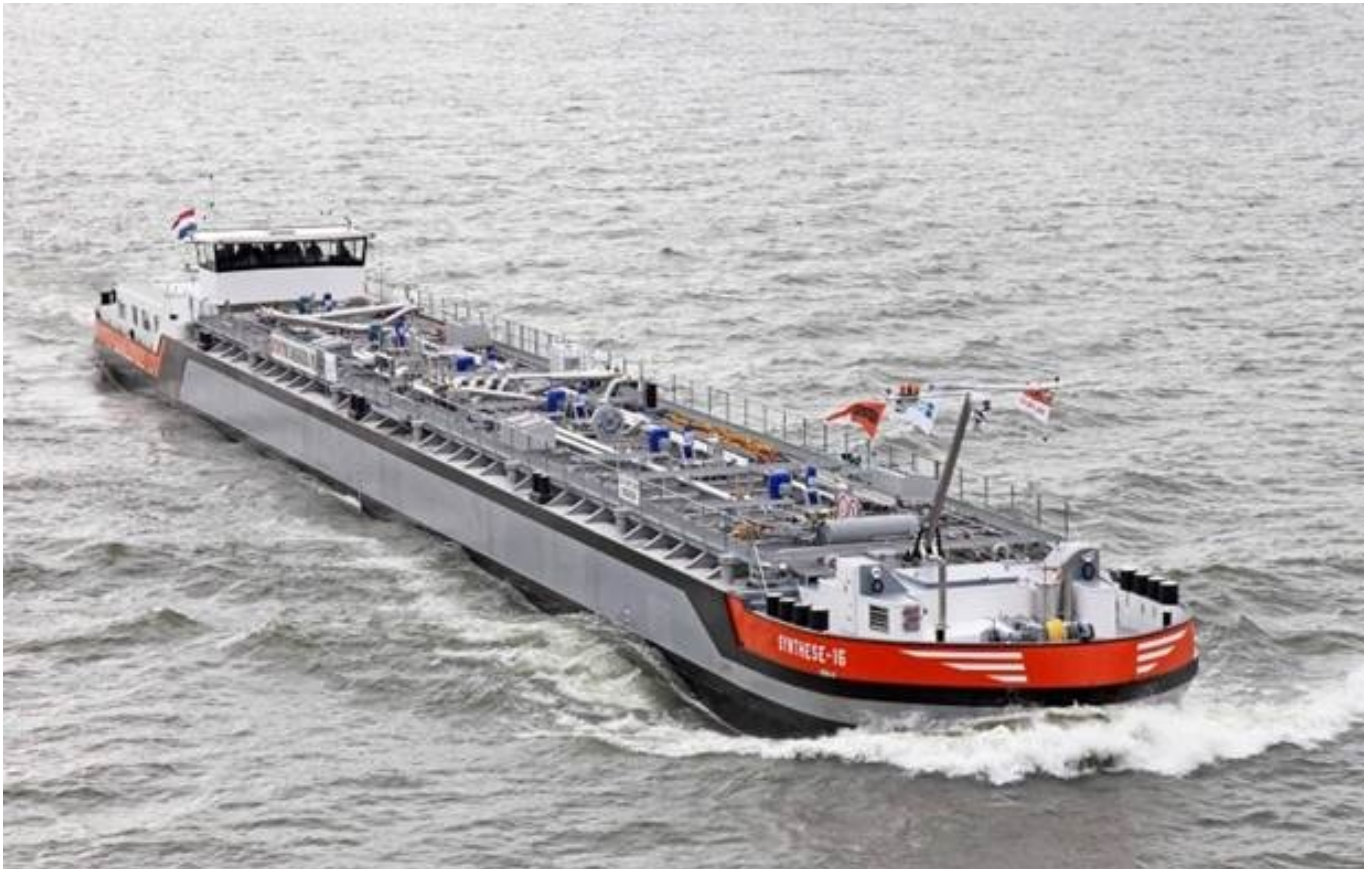
Figure 2: A type-C tank vessel for inland navigation
