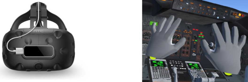
Figure 4.8: Left, Leap Motion mounted on the HTC Vive headset. Right, virtual hands from the Leap Motion
