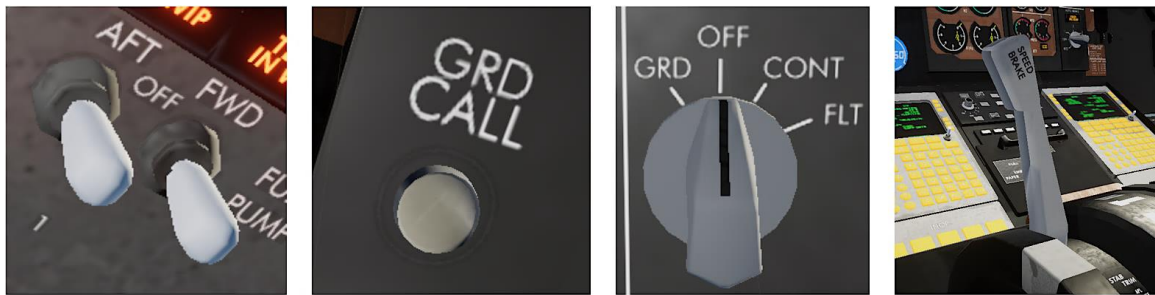
Figure 4.5: Types of controls. From left to right: switches, button, knob and lever
