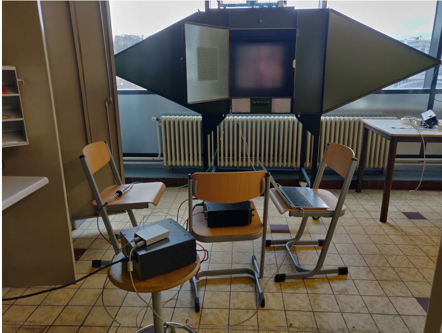
Figure 2.30 – Setup for the wired test in a TEM-Cell (the cell was closed during the tests)
