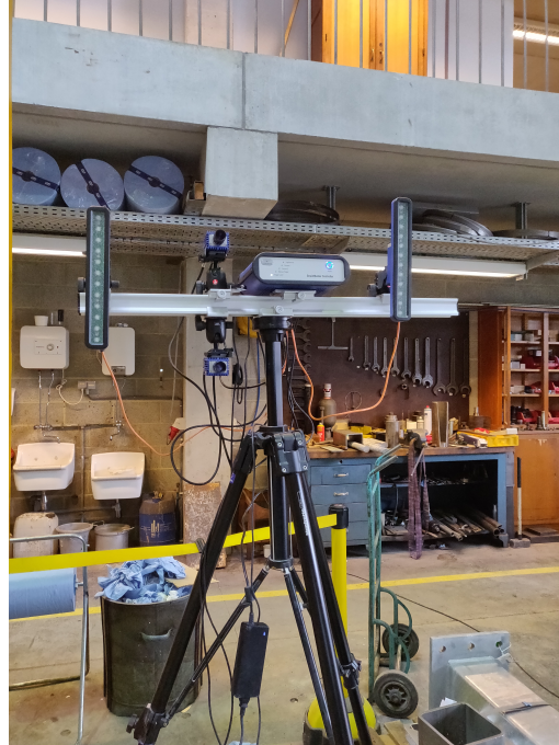
Figure 2.6: Experimental setup of DIC.
