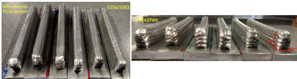
FIGURE 2.16 – Echantillons WAAM de 30 cordons (10 couches)
