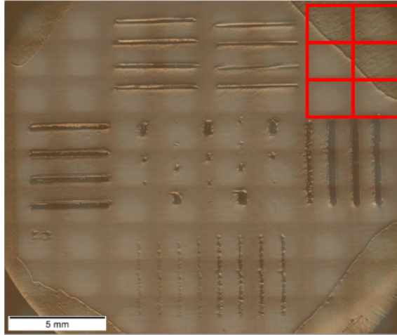
Figure 18: Reconstructed image made of a concatenation of 72 microscopic images. 6 microscopic images are highlighted in red on the top right corner.
