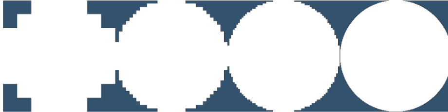
FIGURE 3.1: Pupil shape discretized over respectively 8, 32, 128 and 256 pixels. [13]
