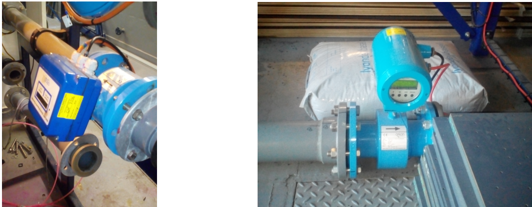
Figure 3.5: Two types of flow meters in the model
