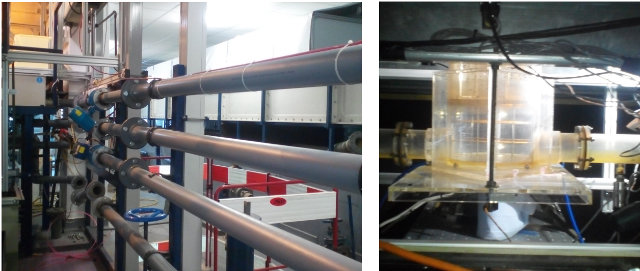
Figure 3.3: Actual experimental facility : upstream pipe system (left) and manhole (right)
