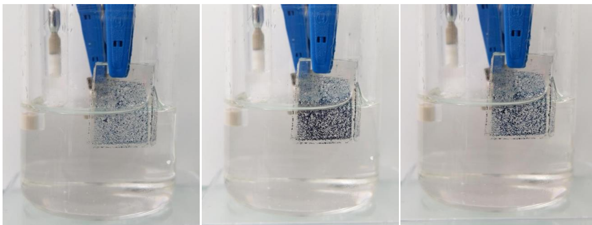
Figure 40: Spin coated MoWO x 1:1 film in the a) as-deposited, b) colored, c) bleached states after thermal treatment at 250°C for 1h.
