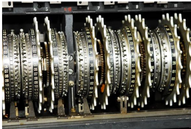
Figure 1.9: The pins of the Lorenz machine either to “on” or “off”.
