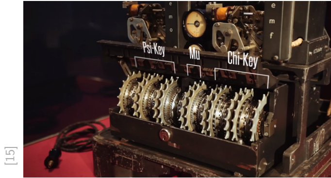
Figure 1.8: The wheels of the Lorenz machine and the keys they produce.
