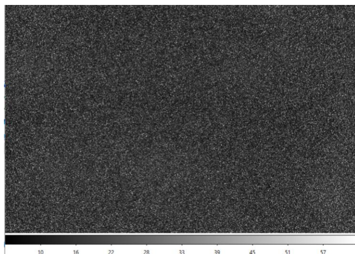
Figure 4.11: Master dark frame in binning 2x2 created with the IRAF task darkcombine.
