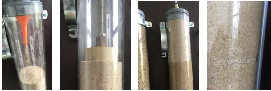
FIG 20: Funnel use, compaction, saturation and observation of the final columns preparation
