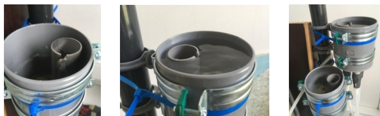
FIG 13: Constant head open overflow devices
