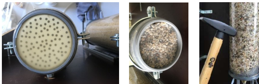
FIG 67 Improvement of second and third trial in column preparation: changes in upper filters and hammer use to help air to exit
