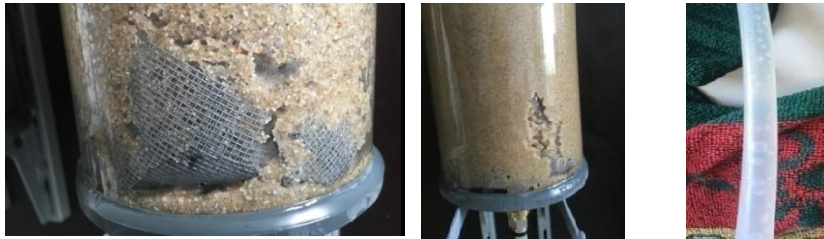
FIG 66 Air bubbles and channels not filled by water in the finer sand samples plus bubbles of air entering the system together with water
