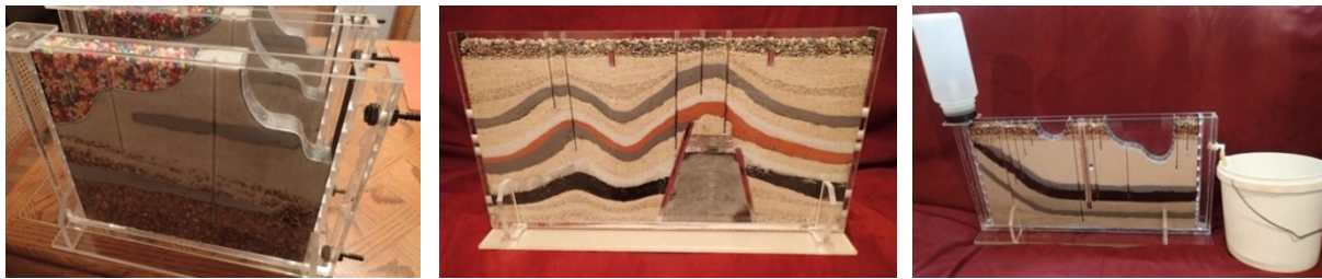
FIG 56 Different examples of 2D physical aquifer model: landfill presence and different geological structures ( https://www.realscienceinnovations.com/groundwater-models.html , consulted in April 2019)
