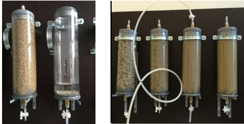
FIG 63 On left side it is shown the column preparation: first layer of water and then sand added; On the right picture the final four columns of the first trial is presented
