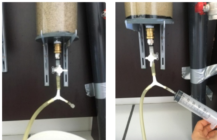
FIG 27 Brief injection of tracer: syringe manually pressed
