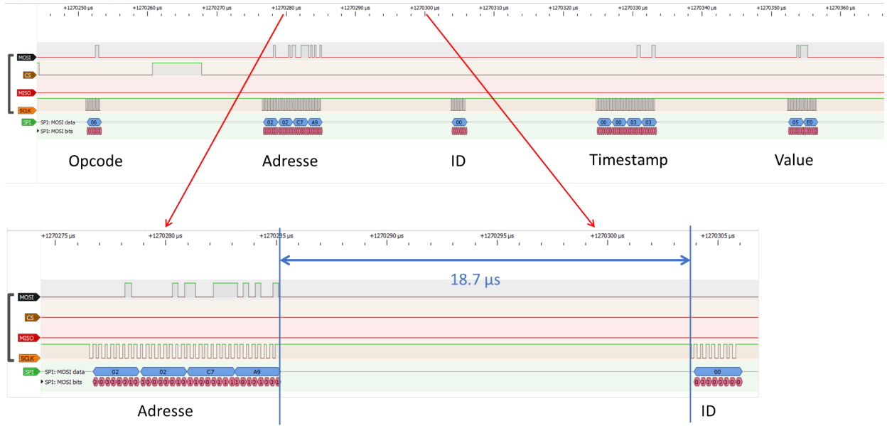
Figure 9.1: Illustration of the delay present when writing measurement obtained by the ADCs in FRAM.
