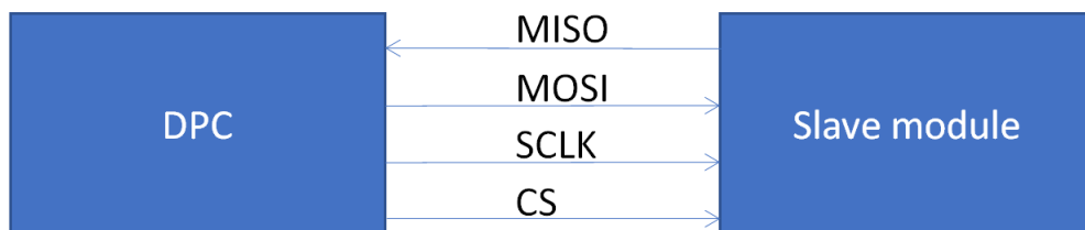
Figure 3.1: Illustration of the wires needed for SPI communication. To communicate with one single module, 4 wires are required: MISO,MOSI,SCLK,CS
