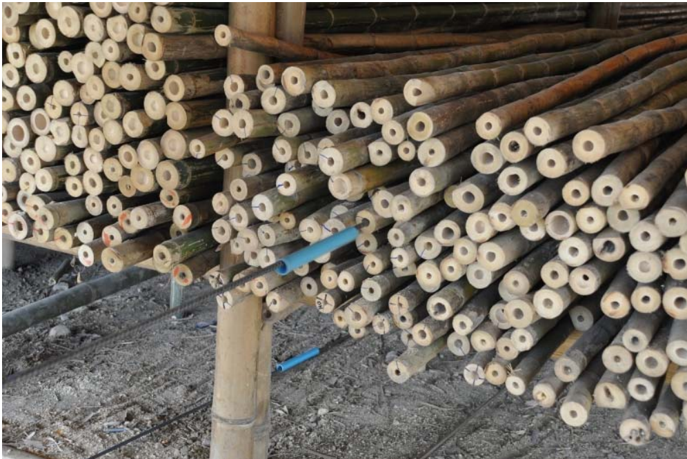
FIGURE 25 - PUNCTURE OF NODAL DIAPHRAGMS
