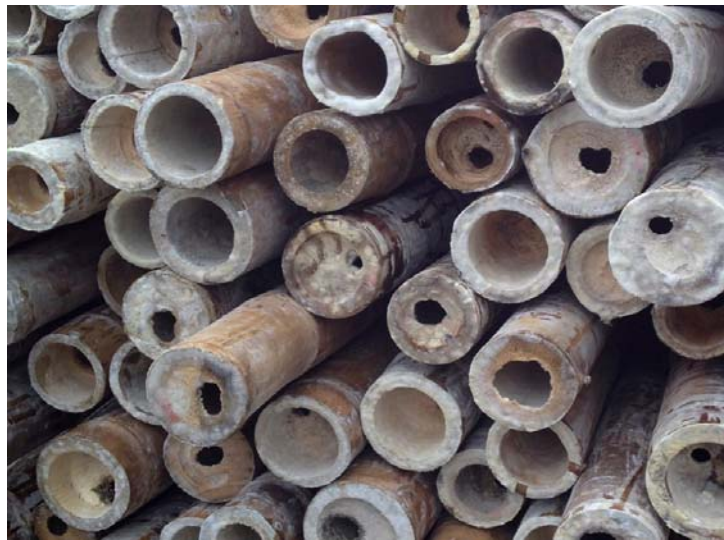
FIGURE 24 - FUNGUS AND ROT ATTACK, ASALI BALI
