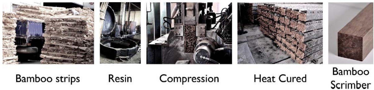
FIGURE 27 - BAMBOO SCRIMBER GENERAL MANUFACTURING PROCESS (SHARMA, GATÓO, BOCK & RAMAGE DRANSFIELD, 2015)
