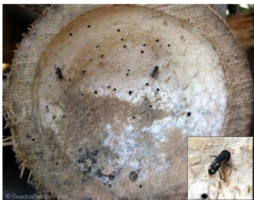
FIGURE 22 - POWDER BEETLE ATTACK, ASALI BALI
