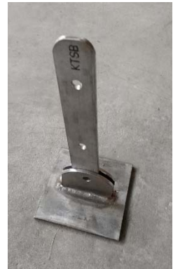
FIGURE 6– METAL PIECE FOR THE FOUNDATION CONNECTION
