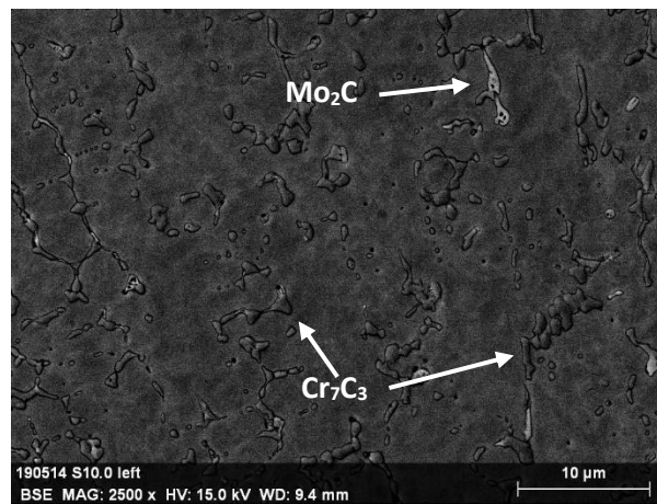
Figure 104: Heat affected zone microstructure on sample S10.0
