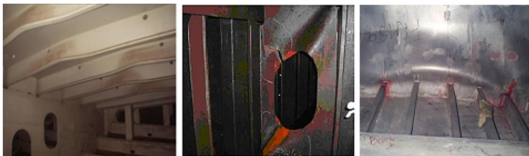
Figure 3: Local structural collapse/Plastic buckling in ship structure [6]
