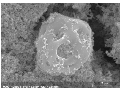
Figure 46 SEM picture of a particle of lignin (light grey) of DPL film sitting on top of carbon beads (dark grey).
