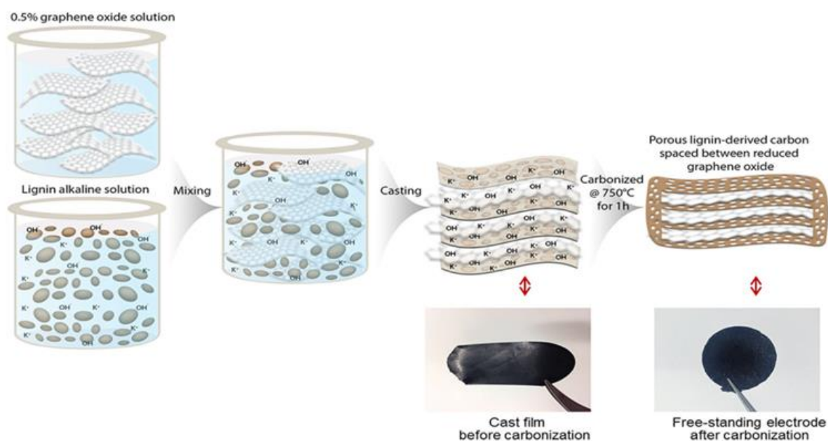
Figure 15 Schematic synthesis of the carbonized lignin-embedded rGO sheets [8].
