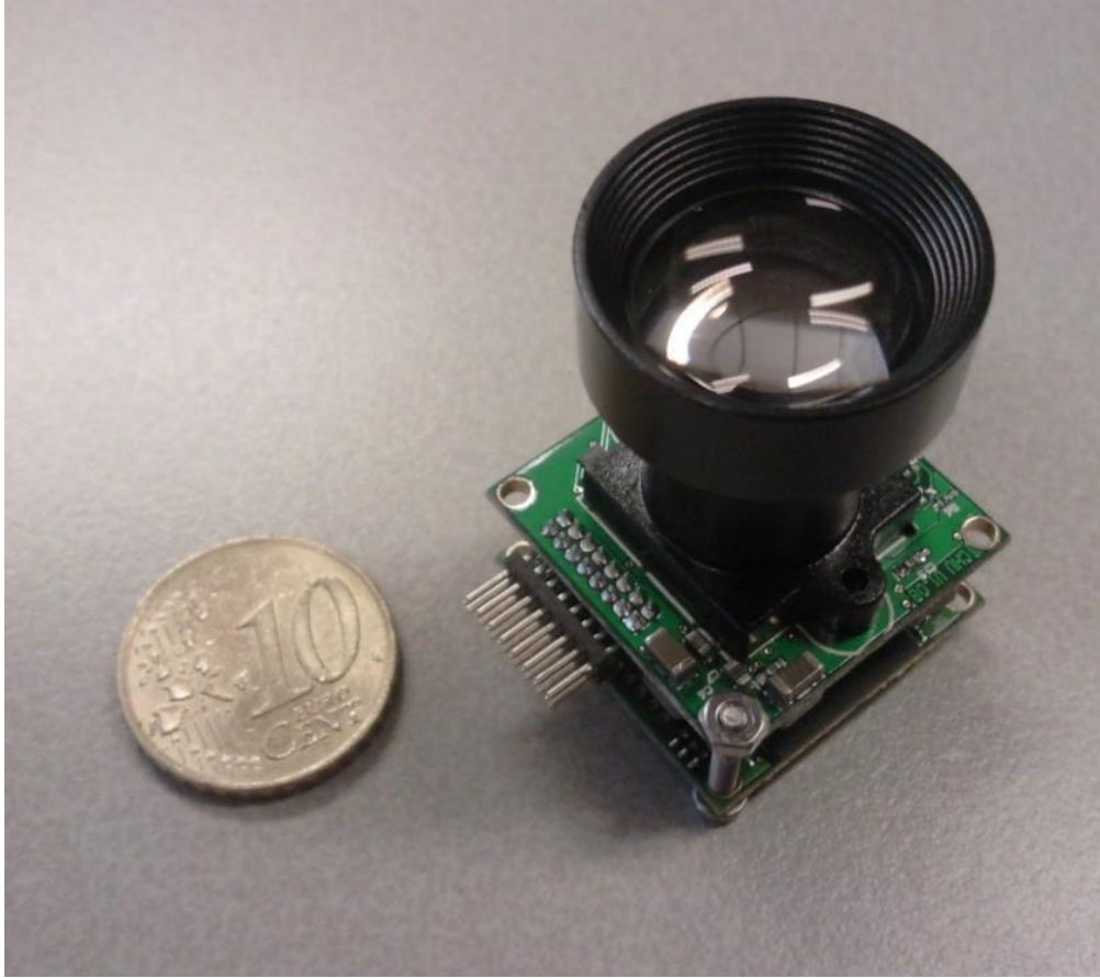
Figure 5.10 ST-200 star tracker by iADCS100 .
