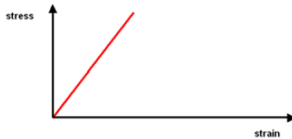
Figure 27 Linear stress-strain relation [6]
