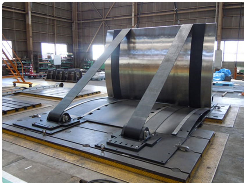
Figure 9 Prototype of the Sea Gate being constructed at MASC, Japan
