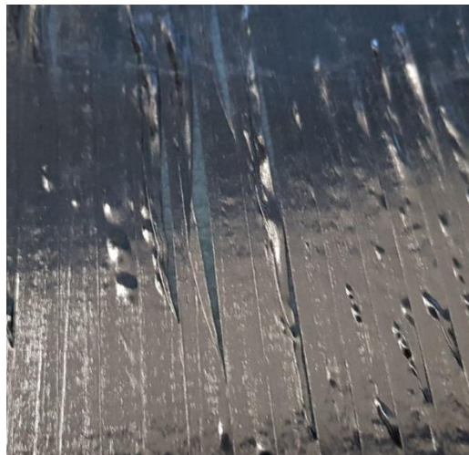
Figure 39 Shrinkage of the tows due to the small radius curvature
