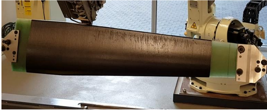
Figure 38 Shrinkage in layer 1, around the trailing edge.
