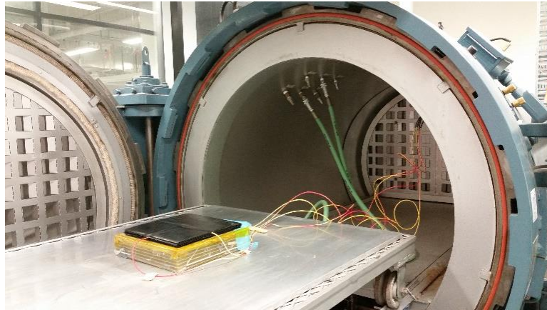
Figure 45 Curing of thick laminate using the proposed curing cycle. (Property of Automated Composites Laboratory, UNSW Engineering)
