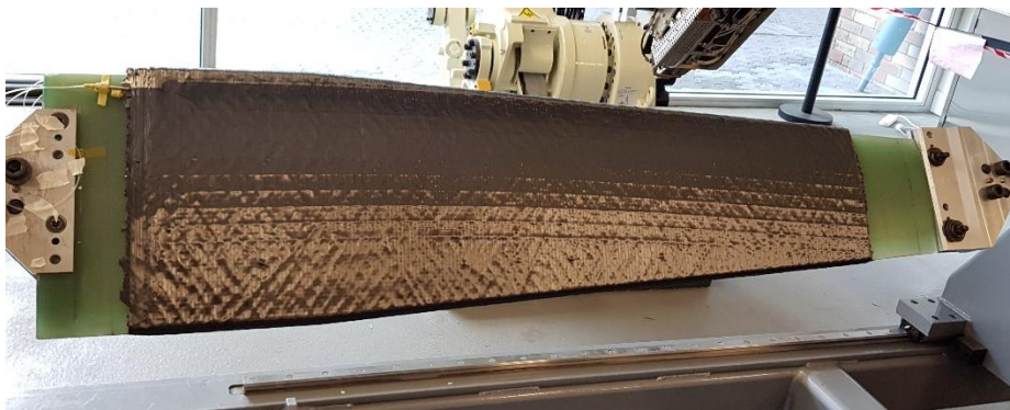
Figure 36 Final layer (96), Full wrapping at 90 Degrees, Mandrel 4
