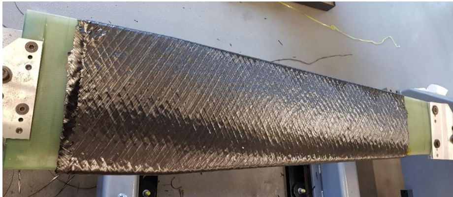
Figure 35 Layer 80, -45 Degrees (Complete surface), Mandrel 4
