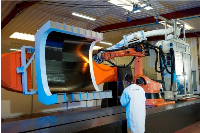
Figure 22 Manufacture using AFP of a section of the fuselage of an Airbus A350, source Coriolis Composites (2015)
