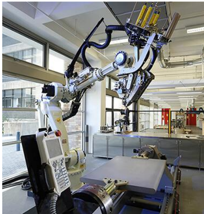
Figure 1 Automated Fibre Placing (AFP) machine at the Advanced Manufacture laboratory, UNSW, Australia (Source: http://advanced-composites.co/facilities_unsw/ )
