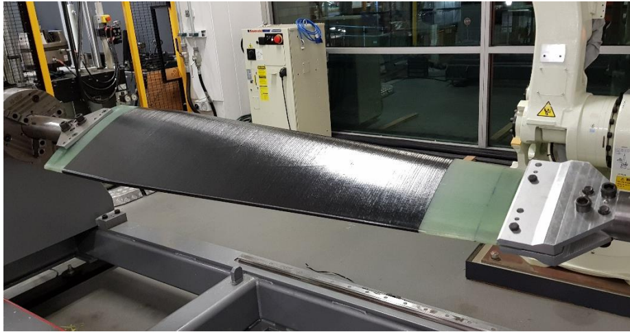
Figure 30 Finish of the first stack of 4 plies at 90 Degrees (Full wrapping)
