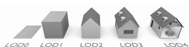
FIGURE 2.2 – CityGML : les 5 LOD (Biljecki (2017), p. 7)
