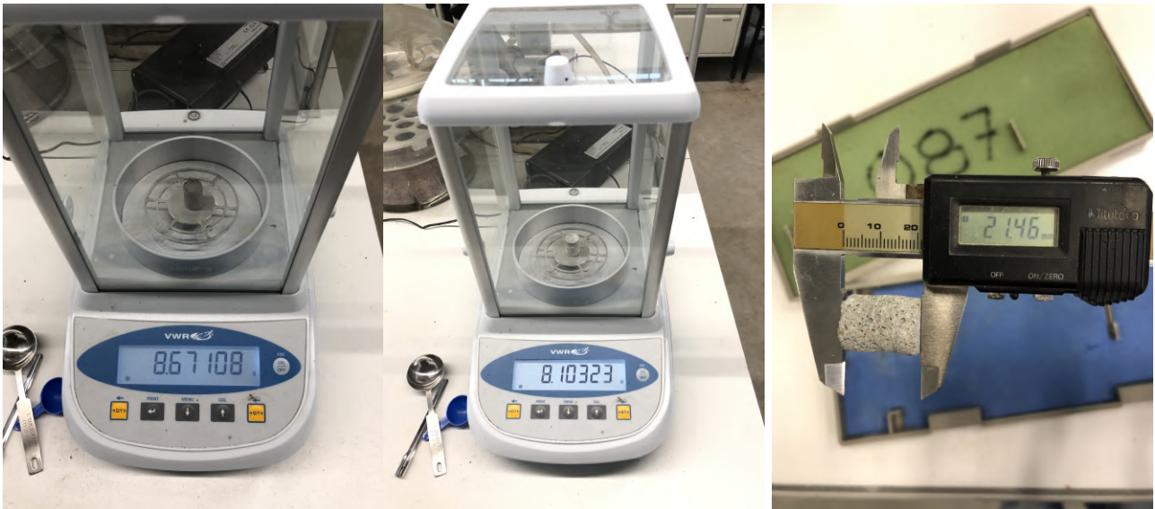
Figure 5.9: Weighing of the sample for the micro-dryer, before (saturated, left) then after the convective drying (partially dried, middle). The sample is also measured after drying (right).
