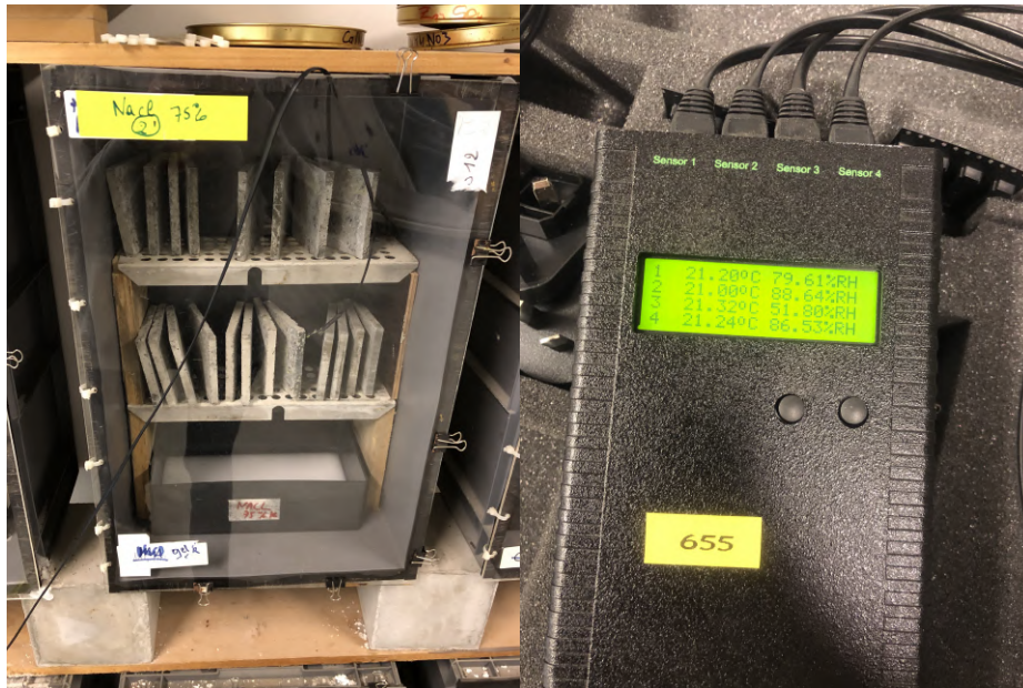
Figure 5.4: Left: Chambers used for the static sorption and desorption experiment, with the RH and temperature probe and the samples inside. Right: sensor housing displaying the measures for the four probes used.
