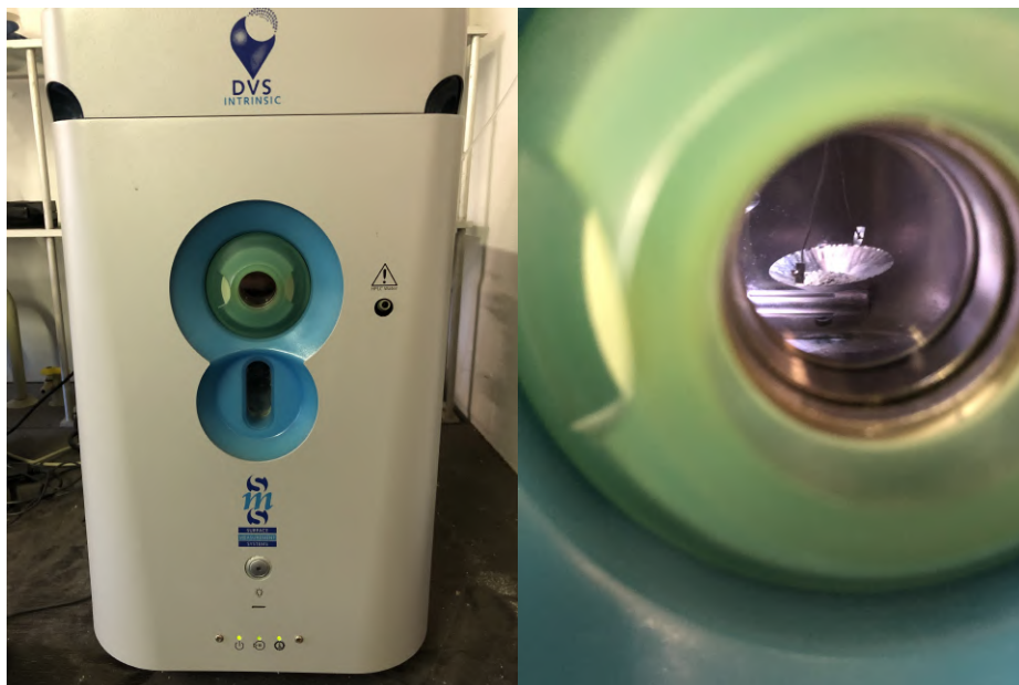
Figure 5.5: Device (DVS Intrinsic) used for the experiment, with the sample inside a little tray.
