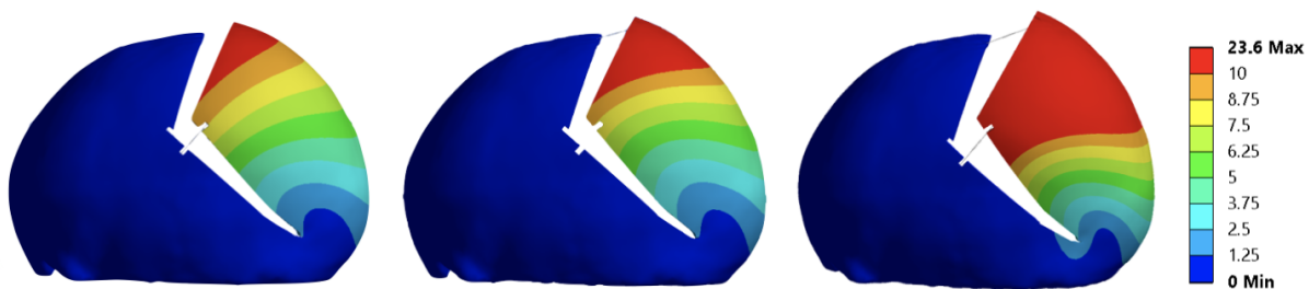
Figure 6.7: Total deformation of the 3 different configurations: spring on the side (left), spring on the top (middle), both springs (right)
