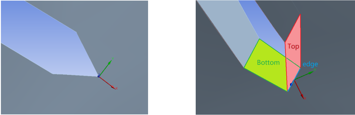
Figure 6.4: Set-up of the crack with the position of the coordinate system and the regions selected.
