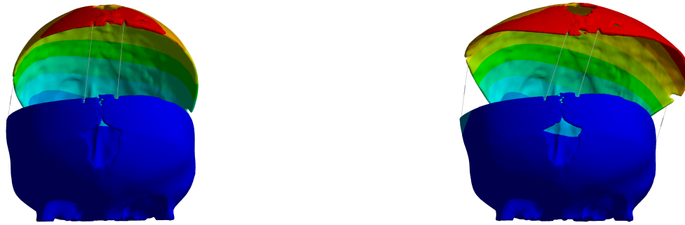
Figure 2.8: Comparison between simulations with linear elements (left) and quadratic elements (right) for patient 3.
