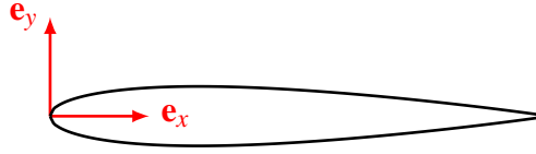
Figure 8.1: Schematic representation the geometry and coordinate system for NACA0012 test case. The vectors \mathbf{e}_x and \mathbf{e}_y are orthonormal vectors.
