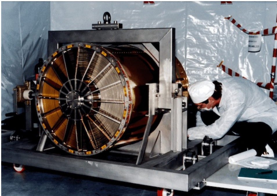
Figure 28: XMM-Newton, 58 nested shells mirrors [41].
