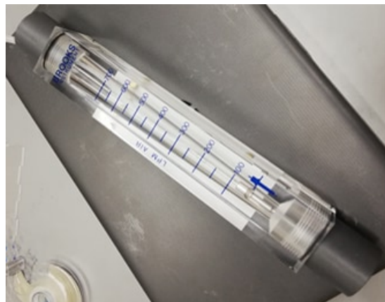
FIGURE 3.10 – Débitmètre "2540I acrylic flowmeter 100-700 LPM of air".
